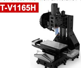
The three-axis screw adopts the central oil cooling and double nut configuration to eliminate the hot extension and reverse clearance of the screw, thus improving the processingaccuracy of the product. As rhe screw rod is fully cooled, the wear caused by heating is reduced, the service life of the screw rod is improved, and the stability of the machine is improved.
